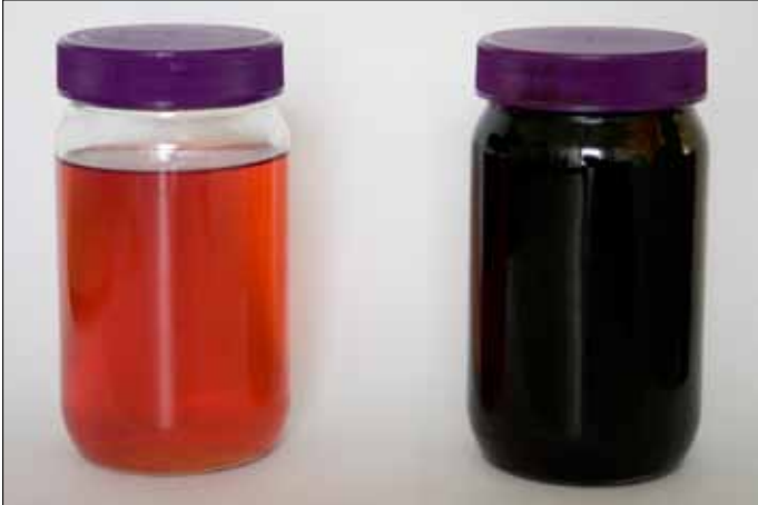
No. 2 oil (left) and No. 6 oil (right). No. 6 oil is the final by-product of the refining process—unrefined sludge.
